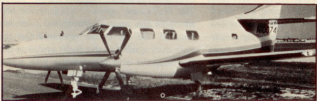
Merlin IIIIC. The Merlin IIIA and IIIB increased in power and weight until the 12,500-pound weight limit for aircraft certificated under Federal Aviation Regulation Part 23 was reached with the IIIB. The Merlin IIIIC and Metro III were certificated under a new set of standards, Special Federal Aviation Regulations Part 41, which is more stringent than FAR Part 23 but less stringent than FAR Part 25, the regulation for transport aircraft. SFAR 41 allows gross weights of more than 12,500 pounds, but sets higher standards for single-engine performance and requires certain safety features, such as engine fire extinguishers. The pilot in command of an SFAR Part 41 certificated aircraft must have a type rating, and two pilots generally are required under these rules. (The aircraft can be operated under FAR Part 23 if gross weight is less than 12,500 pounds.) Most of the differences in the Merlin IIIIC are not readily apparent to the eye. It has a maximum takeoff weight of 13,230 pounds and a maximum cruise of 300 knots.
