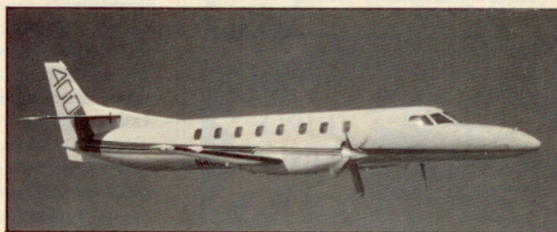
Fairchild 400. The 400, an updated Merlin IV, boasts 347-knot-plus speeds (400 mph) and is powered by two Garrett TPE 331-14 1,100-shp engines turning Dowty Rotol propellers. Certification is expected in late 1985.
