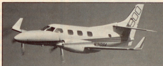
Fairchild 300. Introduced in 1983, replacing the Merlin IIIIC, the 300's major distinguishing feature is a new pair of winglets, designed to reduce spanwise airflow and drag. Garrett 900-shp engines supply the power. Maximum speed is 300 knots.
